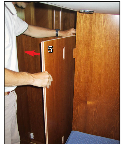
5- Dismantle the back of the hanging locker.
