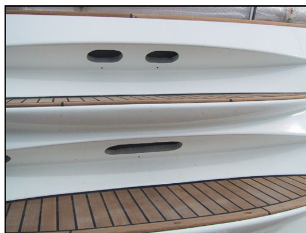
Engine compartment air intake and exhaust
