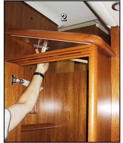
2 - Dismantle the top of the hanging locker (bolt).
